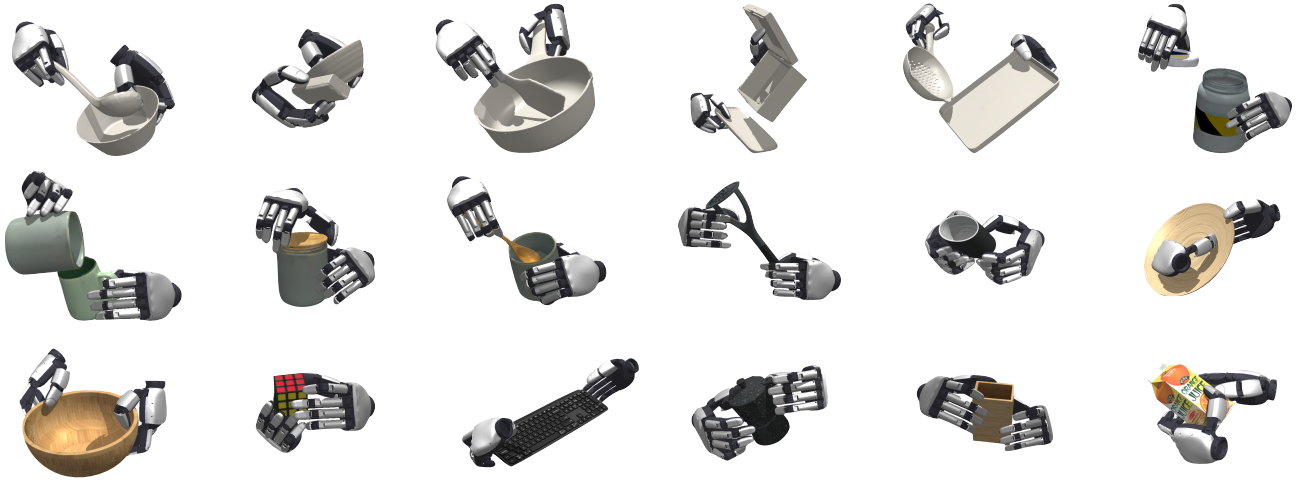
Fig. 3. Qualitative retargeting results. Representative snapshots of dexterous robot manipulation generated by FlashDexRetarget in simulation. The examples span tool use, container handling, and manipulation of everyday objects, illustrating the variety of object geometries and hand-object configurations covered by the retargeted motions.
