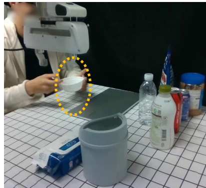
Figure 19: A task-predictor input frame during the eating phase: the user eats cereal while the milk and cereal are already in storage. Here the FSM predictor outputs NO_ACT while the list predictor fires T2 (Milk → Person).
